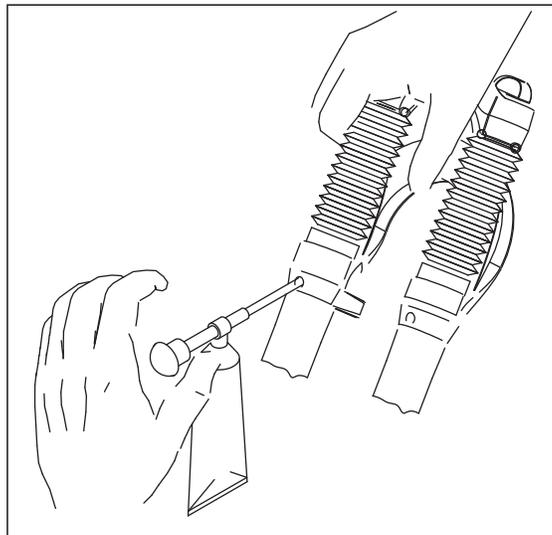
**IMPORTANT:** When filling the fork with grease through the Microlube grease ports it is important to note the grease is being forced between the upper and lower bushing (Figure 7). If the area is over-filled, the force of the grease may force the upper bushing and dust seal out.
